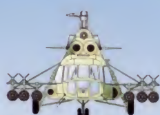
Mi-8 'HIP-E': Probably the most heavily armed helicopter in service, the 'Hip-E' carried up to six pods of 32 rockets.
